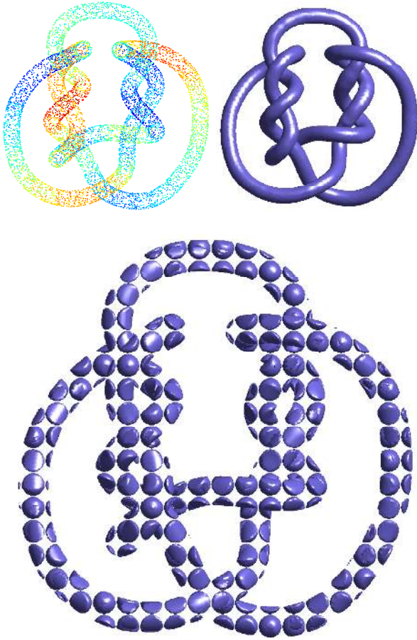
Figure 6. An example using the “knot” data set consisting of 10K data points in three dimensions, as shown on the top left (the colours have no special meaning). The implicit surface rendered on the top right was constructed using approximately 5K basis functions. The lower image demonstrates that set operations such as intersection are trivial with implicit shape definitions, regardless of the topological complexity that results – we intersected the knot shape with a grid of balls (also defined as an implicit).
