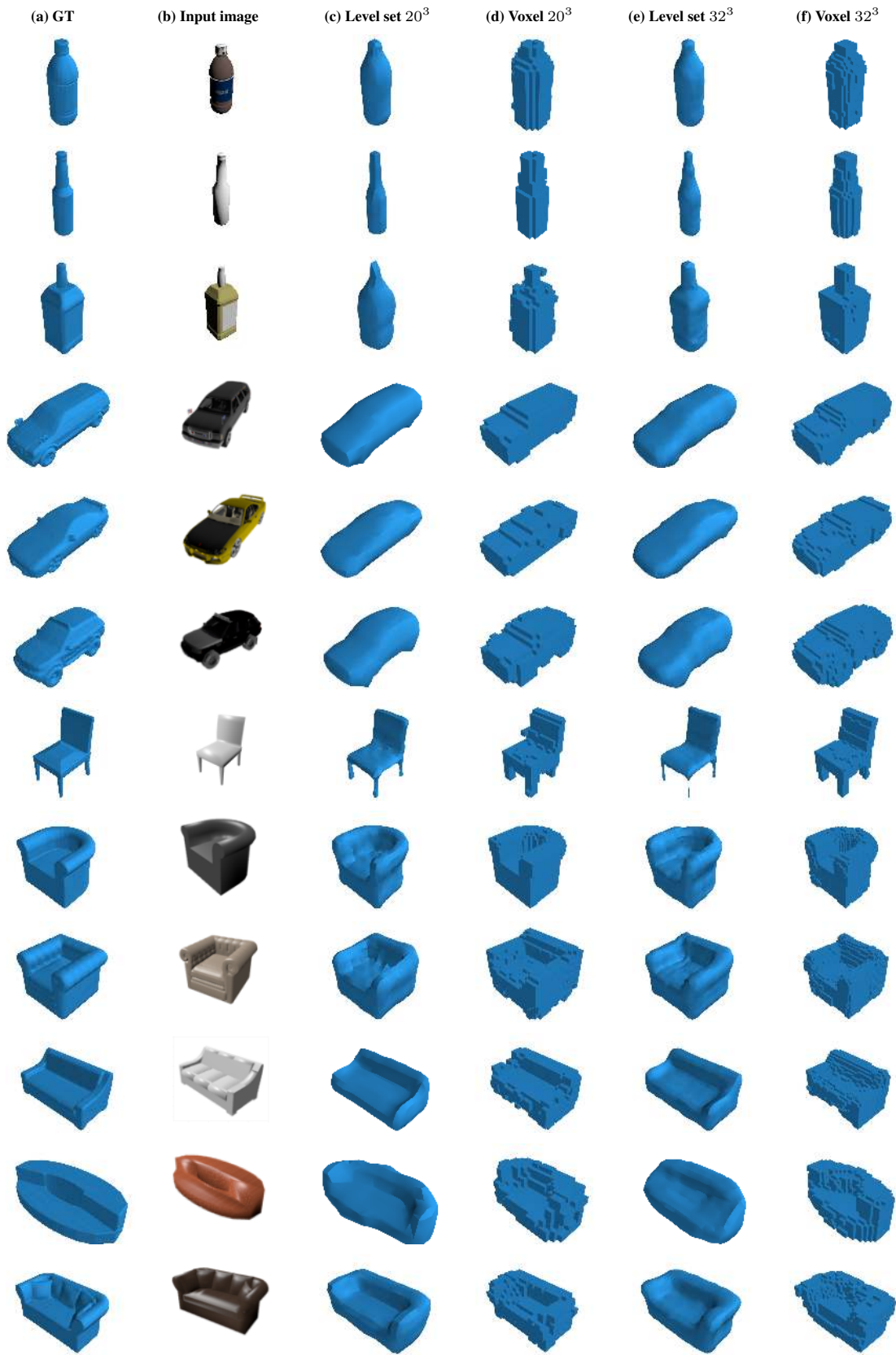
Figure 4. 3D shape inference from a single 2D image. The columns are (a) ground-truth shape, (b) input image, (c) predicted shape, level set, 20^3 , (d) predicted shape, voxels, 20^3 , (e) predicted shape, level set, 32^3 , (f) predicted shape, voxels, 32^3 .
