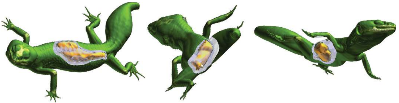
Fig. 9. Visibility preserving importance compositing (VPImC). The dataset is shown under different viewpoint settings with constant visibility of the focus object which is independent from the thickness of the occluding context part.
