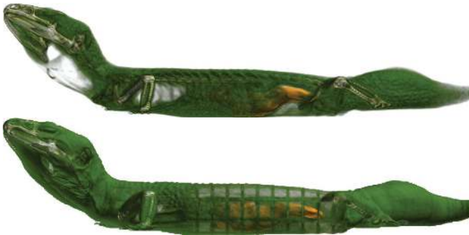
Fig. 3. Comparison between traditional volume rendering (top) and importance-driven volume rendering (bottom). The orange inner organ is the focus object
