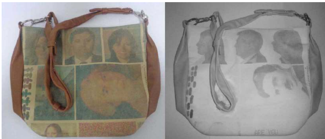
Figure 8. Safety print on leather product, visual image left, Z image, right (courtesy dr. J. Žiljak)
