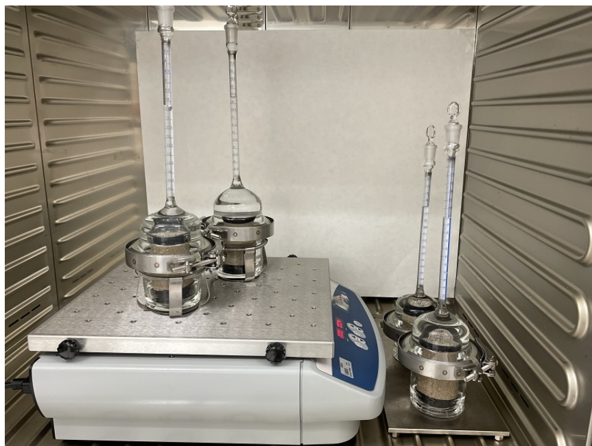
Figure 5: Two pairs of core plugs in the modified Amott cells are tested at constant shaking (left cells mounted on the shaker platform), and at static conditions (right cells).
