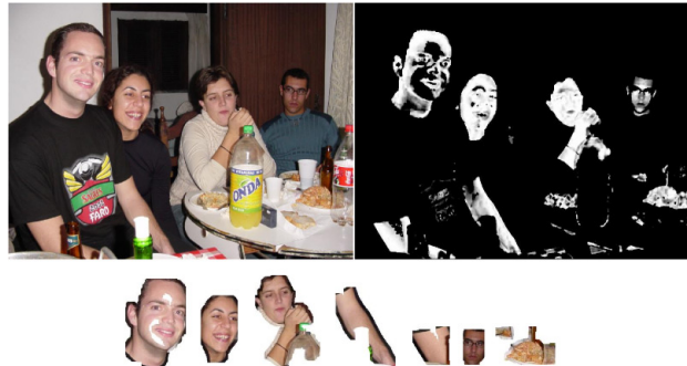
Fig. 4. Very complex picture with different sizes groups of skin. Showing the original image, the median image and the group resulting analysis. Only one group is not correctly classified since it have a very similar color to skin (food in table). The grouping algorithm also connects two separated elements (forehead from the rest of the face) that compose the man with glasses. Image size: 800x600. Input device: Sony P51. Comments: Night picture with flash, indoor.
