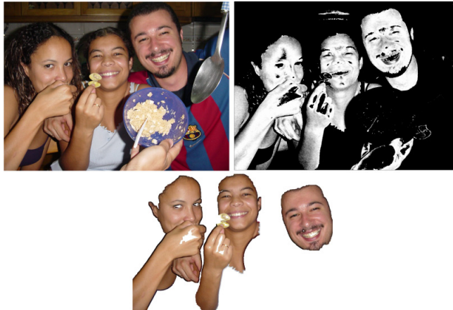
Fig. 6. Small complex background with frontal different color skin faces. Showing the original image, the median image and the group resulting analysis. One white Caucasian and two white-dark skin descents are present. The neck was discarded because it possesses a small number of pixels. Image size: 800x600. Input device: Sony P51. Comments: Daylight with artificial light, indoor.
