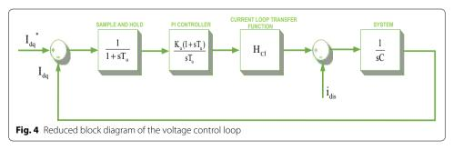
In the symmetrical optimum method, open loop transfer function is approximately symmetrical at the crossover frequency ( $\omega_c$ ). The relationship between  $\omega_c$  and phase margin is given in Eq. (22).
