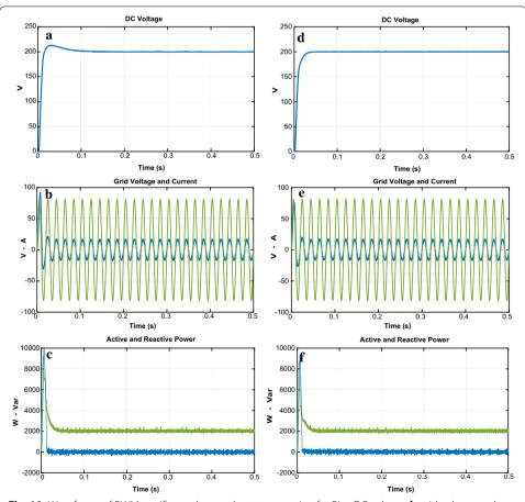
**Fig. 10** Waveforms of PWM rectifier under steady state operation for Pl. **a** DC voltage, **b** grid voltage and current, **c** active and reactive power, for NFC, **d** DC voltage, **e** grid voltage and current, **f** active and reactive power
