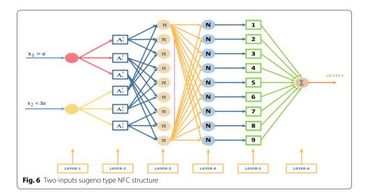
and  $e = V_{dc}^*(k) - V_{dc}(k)$ ) and the change of error ( $\Delta e = e(k) - e(k-1)$ ) are chosen for NFC that used in control method.  $\Delta V_{dq}$  and  $I_d$  are obtained from the output of NFCs. At the control method, two units of NFC that shown in Fig. 6 were used totally which one is for control of DC bus voltage and the other one is for control of dq-axis currents.
