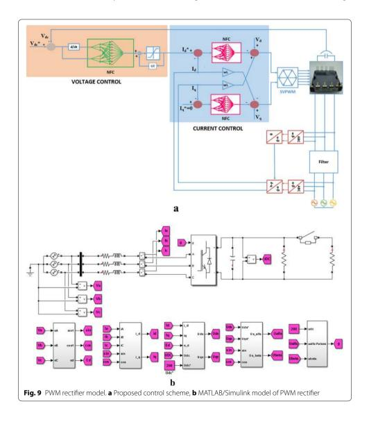
and dq-axis currents of PWM rectifier are controlled by using NFC controllers. Also, the simulation model has designed in MATLAB/Simulink environment as shown in Fig. 9b. The transformation blocks used in the simulation model is also given in Fig. 9b.
