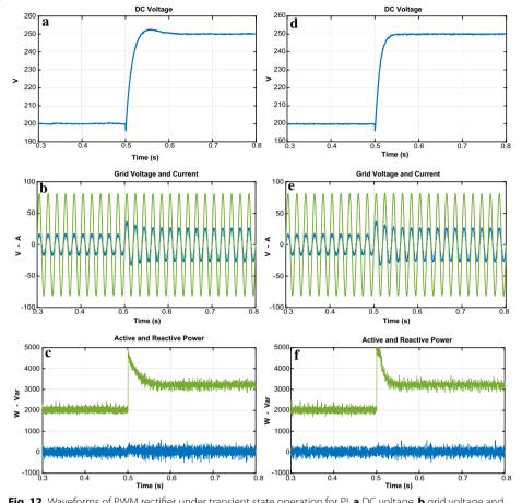
**Fig. 12** Waveforms of PWM rectifier under transient state operation for Pl. **a** DC voltage, **b** grid voltage and current, **c** active and reactive power, for NFC, **d** DC voltage, **e** grid voltage and current, **f** active and reactive power
