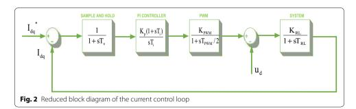
where,  $T_{\rm et}=4T_{\rm ei}\zeta^2$ ,  $\xi=\sqrt{2}/2$ ,  $T_{\rm et}=2T_{\rm ei}$ . The performance of the PI controller designed for the control of dq-axis currents is examined by using the reduced block diagram of the control loop (Blasko and Kaura 1997). As it is shown in Fig. 3, the time constant of the PI controller is selected as  $T_{\rm i}=10T_{\rm ei}$  and  $T_{\rm i}=T_{\rm RL}$ . Also, the responses of PI controllers are shown in Fig. 3.
