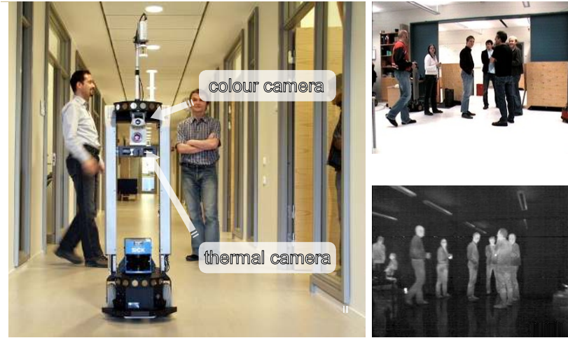
Figure 1: ActivMedia PeopleBot robot equipped with a thermal camera and a standard camera (left). Example of an image from the colour camera (right-top) and thermal camera (right-bottom).
