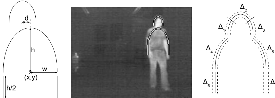
Figure 2: The elliptic measurement model for thermal images. Model parameters are shown on the left. Division of ellipses into 7 regions is shown on the right.
