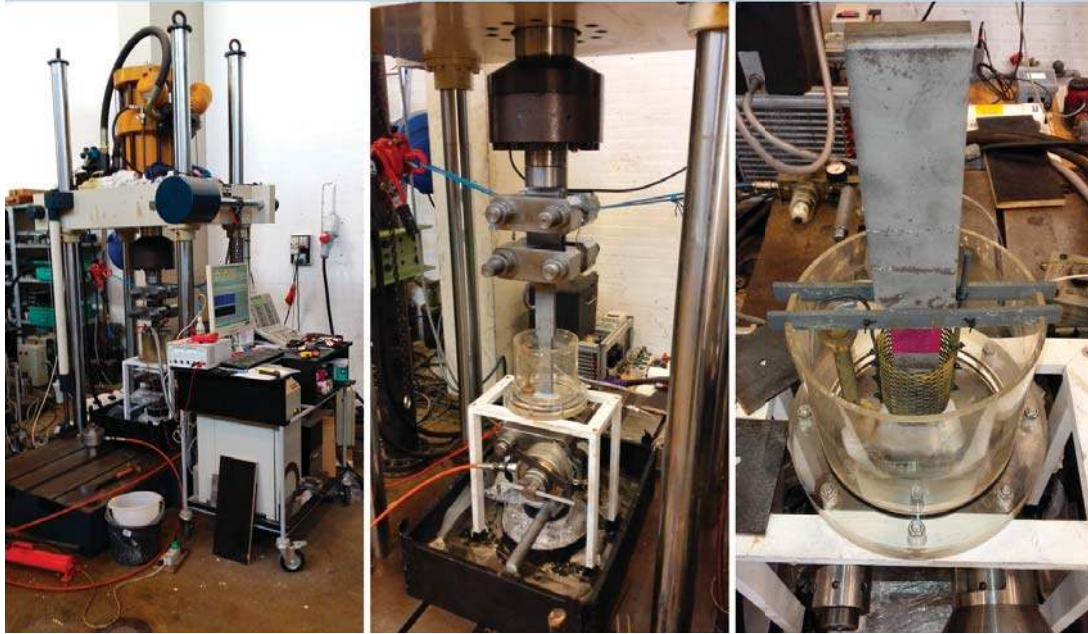
Figure 5.10: Corrosive environment test setup
