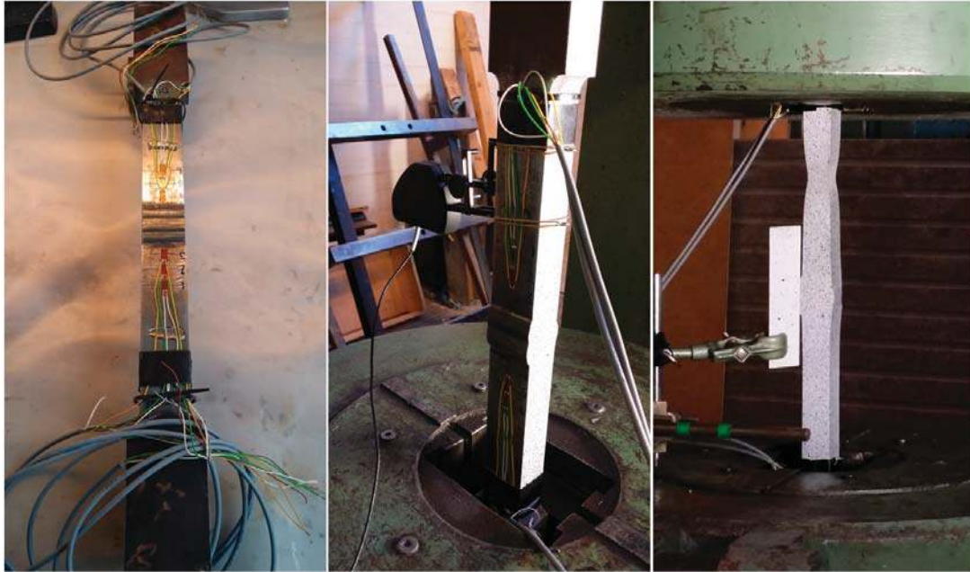
Figure 4.17: (Left) Strain gauges location and preparation, (center) prior to static testing, measurement equipment setup and (right) visible surface pattern for the DIC system and necking of the specimen occurring above the weld
