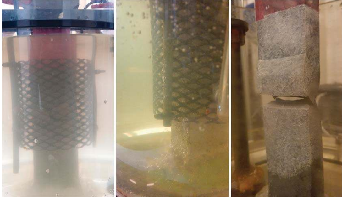
Figure 5.13: Calcareous coating formation on the corrosion fatigue specimens
