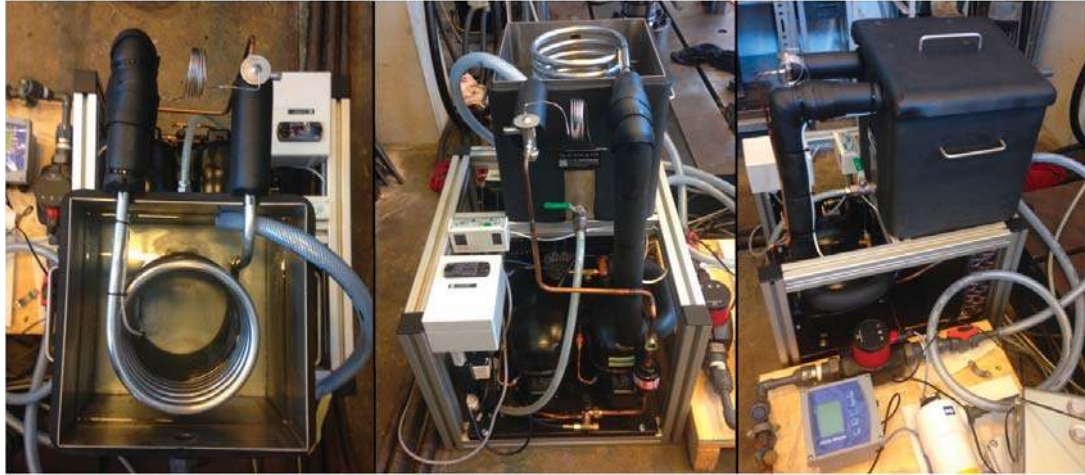
Figure 5.2: Cooling system for the corrosion environment, [12]
