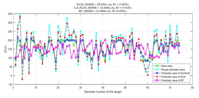
Figure 11. The comparison of the prediction results of the Z-axis errors of the test set target.
