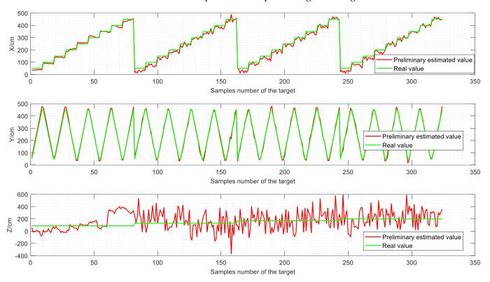
sensitive. Therefore, it is indispensable that the *Z*-axis coordinates errors compensation is carried out to accomplish accurate positioning of the target.
