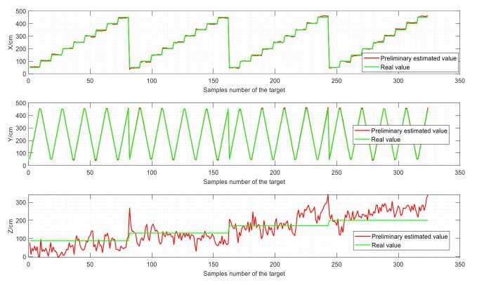
**Figure 9.** The comparison of the true value and estimated value of the target coordinates without signal interference.
