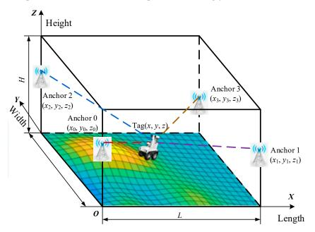
Figure 1. Schematic diagram of the principle of TOF-based UWB data collection.
