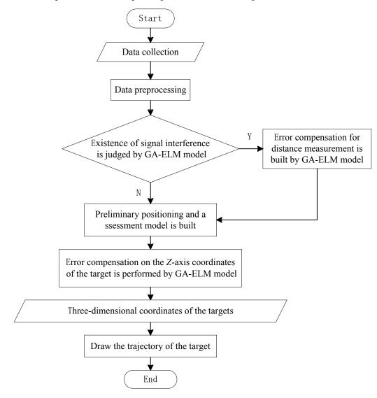
Figure 2. Workflow chart of the overall method.
