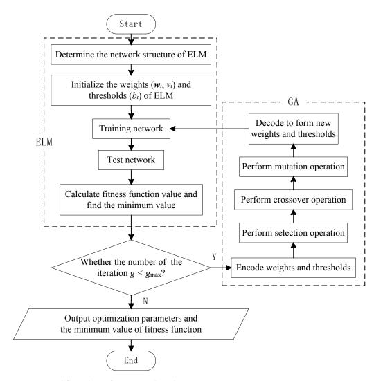
Figure 4. Workflow chart of GA-ELM algorithm.
