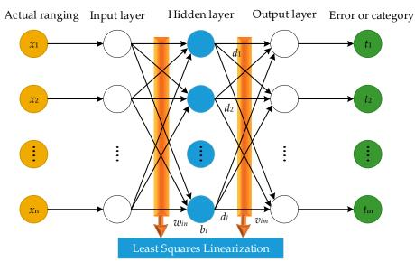
Figure 3. The network topological structure diagram of ELM based on least squares linearization.
