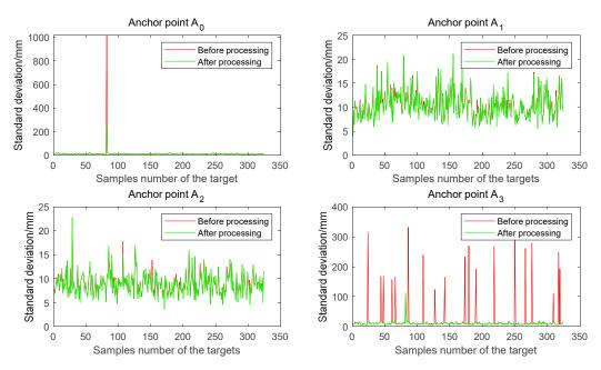
**Figure 5.** The standard deviation comparison of the samples before and after processing without signal interference.
