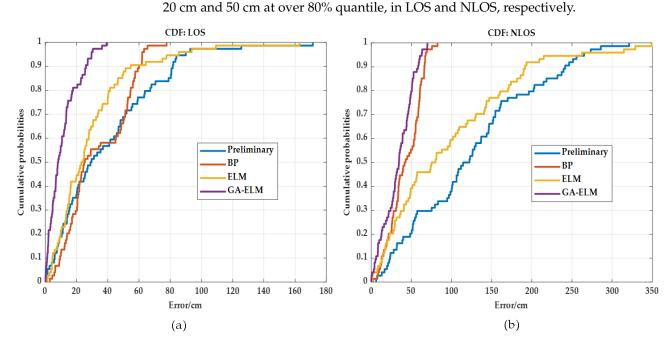
**Figure 15.** The comparison of CDFs for different algorithms under LOS and NLOS: (**a**) Without signal interference; (**b**) With signal interference.
