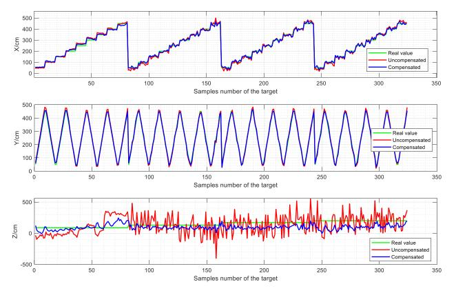
Figure 13. Comparison before and after ranging errors compensation with signal interference.
