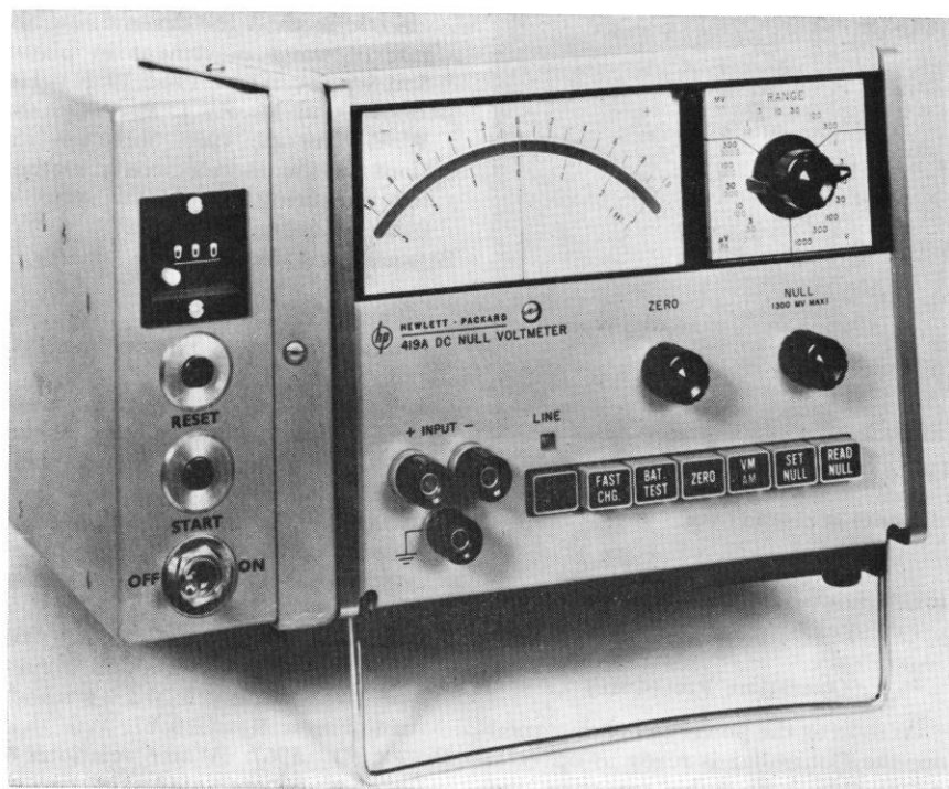
Fig. 1. Microvoltmeter with heat pulse and timing circuits in box attached to side.
