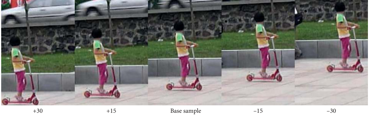
FIGURE 3: Cyclic shift of the target sample. Taking the target image as the base image, the method of cyclic offset can get some approximate negative samples as training samples.
