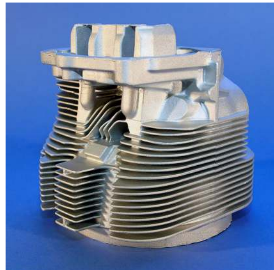
Fig. 9 General aviation cylinder head produced from Al-Ce binary alloy
