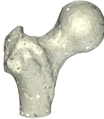
Figure 14: RFS-mesh smoothed by the HC-algorithm in combination with edge swapping.
