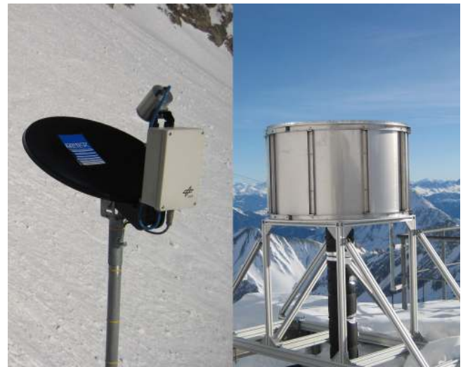
Fig. 1. Micro Rain Radar 2 (MRR) (left) and MIRA35 cloud radar (right) at the UFS Schneefenerhaus.
