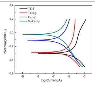
FIGURE 3 | Potential dynamic polarization curves of TC4, TC4-p, CaP-p, and Sr-CaP-p.
