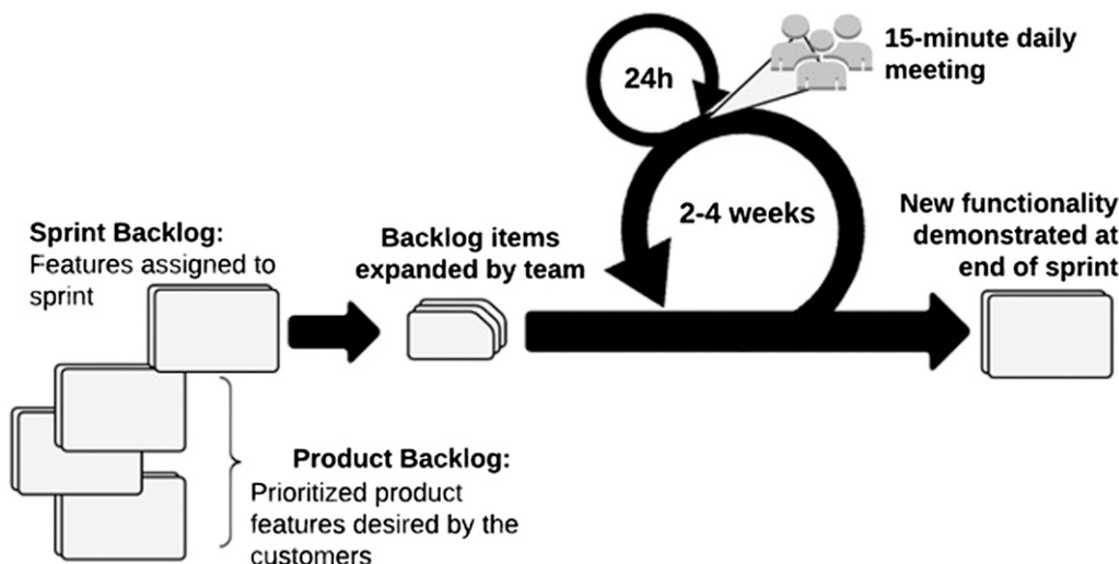
FIGURE 1. The Scrum process model (adapted from Boehm and Turner 2005)
