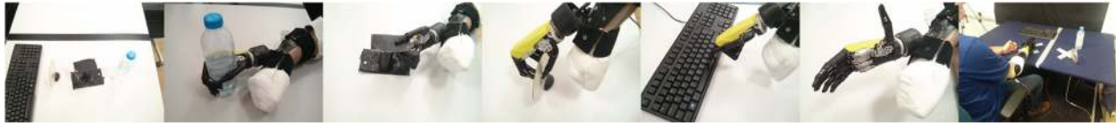
Fig. 3 Real-time control pick and place experiment. Participants were instructed to use a prosthetic hand to grasp and relocate three objects and finally press the 'space' key on a computer keyboard (left). Five grip types were used: power/cylindrical (water bottle), lateral (credit card simulator), tripod (CD), index finger pointer (computer keyboard) and hand open. A trial with an amputee participant is shown on the right
