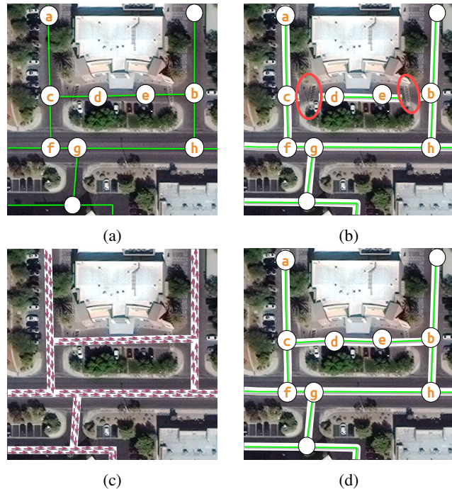
Figure 1: Road network extraction formulated as binary segmentation fails to produce topologically correct road map due to change in road appearance. (a) Annotators trace lines (highlighted nodes) along the center of roads with a traversable shortest path (a, c, d, e, b) for a \rightarrow b . (b) Fragmented road network estimated using segmentation resulting in path (a, c, f, g, h, b) for a \rightarrow b . (c) Tracing roads with orientation to achieve connectivity. (d) We extract connected and topologically correct road networks using segmentation and orientation.
