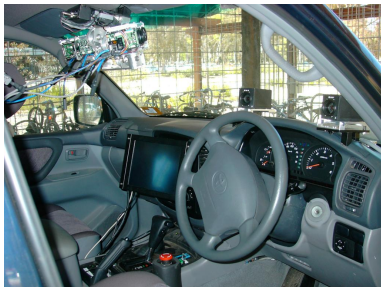
Fig. 1. The ANU/NICTA/CSIRO Intelligent Vehicle. The cameras are mounted where the rear view mirror would be.
