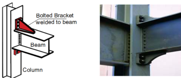
Fig. 5. Bolted bracket and typical connection
