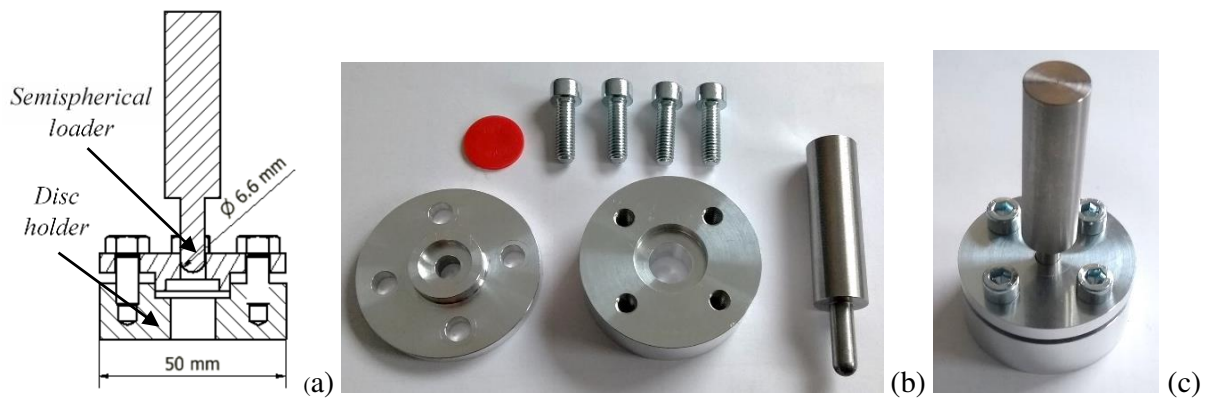
Figure 5. Small punch test cross-sectional drawing – units in mm (a), parts of the device (b) and mounted device (c)
