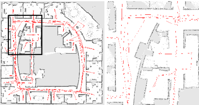
Fig. 4. The Intel Research Lab. The robot starts in the upper part of the circular corridor, and runs several times around the loop, before entering the rooms. The left image depicts the resulting map generated with 15 particles. The right image shows a cut-out with 1\text{ cm} grid resolution to illustrate the accuracy of the map in the loop closure point.
