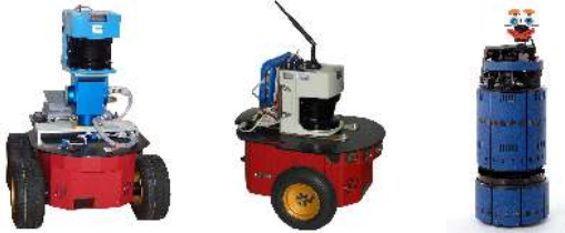
Fig. 3. Different types of robot used to acquire real robot data used for mapping (ActivMedia Pioneer 2 AT, Pioneer 2 DX-8, and an iRobot B21r).
