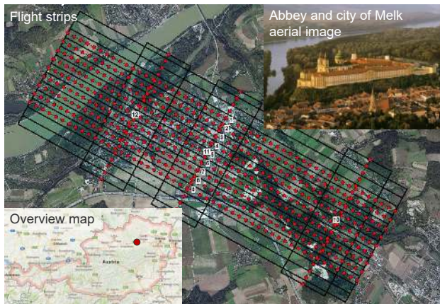
Figure 4. Study area city of Melk (Austria), center: planned flight trajectories (black lines) and camera positions (red circles), upper right: aerial image of the abbey and city of Melk, bottom left: location of study area (red circle) within Austria
