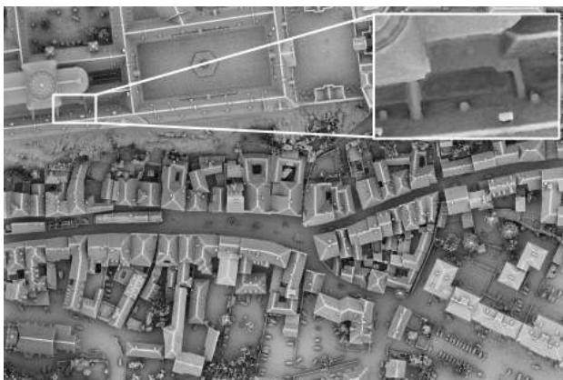
Figure 9. Ambient occlusion shading of hybrid LiDAR-DIM DSM mesh; detail: narrow alley within the abbey with roof points stemming from DIM and ground floor points from LiDAR
