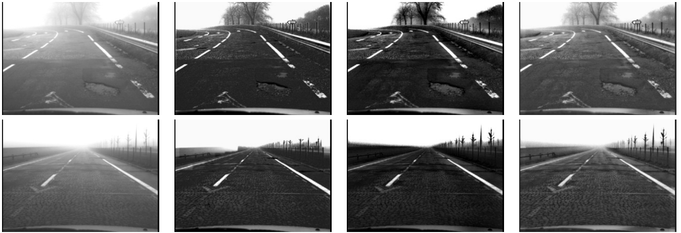
Fig. 1. From left to right, the original image with fog, the results obtain with visibility enhancement using [5], [6] and [1] algorithms. Notice how the road close to the vehicle is over-contrasted or too dark.
