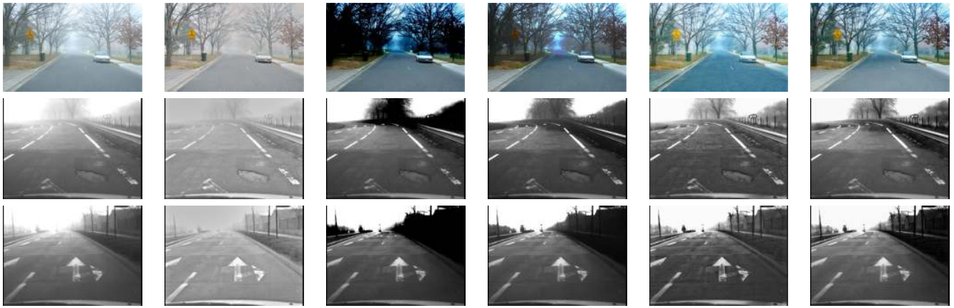
Fig. 2. From left to right, the original image with fog, the images enhanced using algorithms: retinex, planar assumption with clipping, free-space segmentation, no-black-pixel constraint and no-black-pixel constraint combined with planar assumption.
