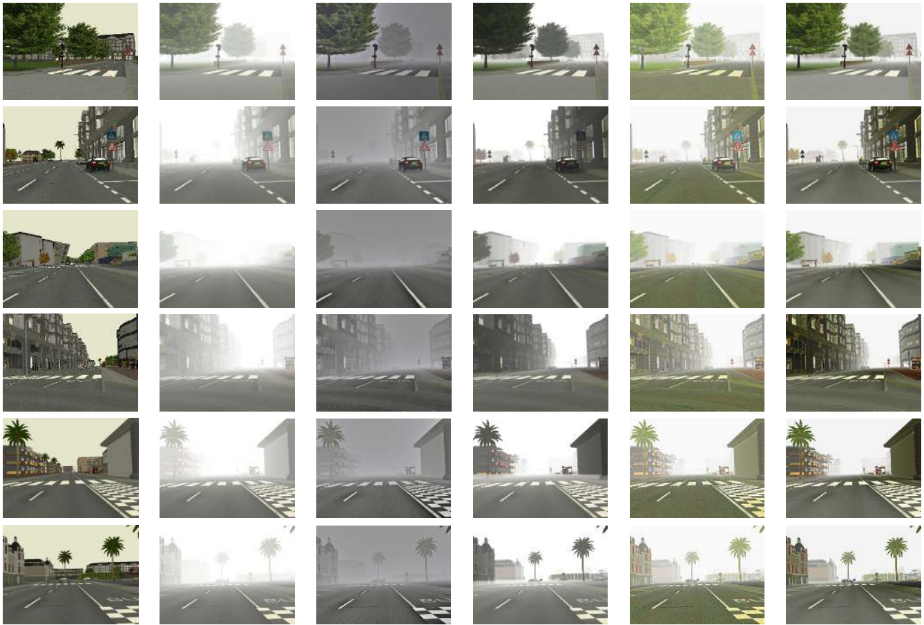
Fig. 5. From left to right, the original image without fog, the processed image with uniform fog, the images enhanced using multiscale retinex, free-space segmentation, no-black-pixel constraint and no-black-pixel constraint combined with planar scene assumption.
