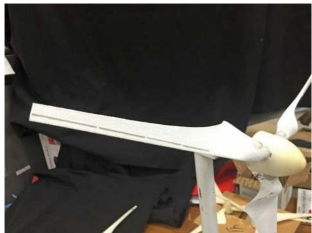
Fig. 1 The slotted wind turbine blade fabricated and tested at UWM Wind Tunnel
