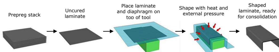
Figure 1. Illustration of composite vacuum forming process.
