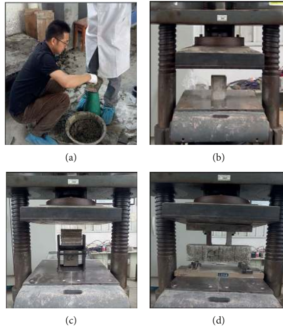
FIGURE 2: (a) Slump test, (b) compressive test, (c) splitting tensile test, and (d) flexural strength test.
