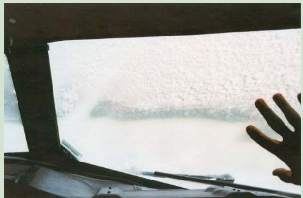
FIG. SBI. Ice accumulates on the windshield of the NOAA P-3 aircraft during the 18 Dec 2001 IMPROVE-2 research flight.
