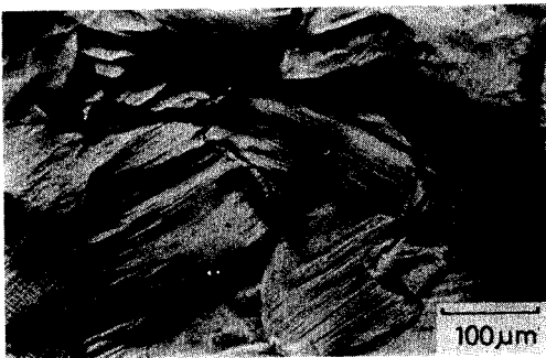
Photo.4 Surface slip markings of 0.1% boron added \text{Ni}_3\text{Al} tested in tension to the fracture point.
