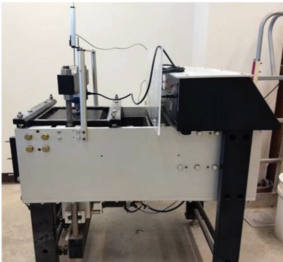
Figure 6.2 Large-scale direct shear machine manufactured by GeoComp.
