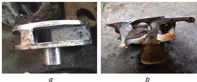
Fig. 1. Ground pump impeller 8Gr-8: a – new impeller; b – worn-out impeller
