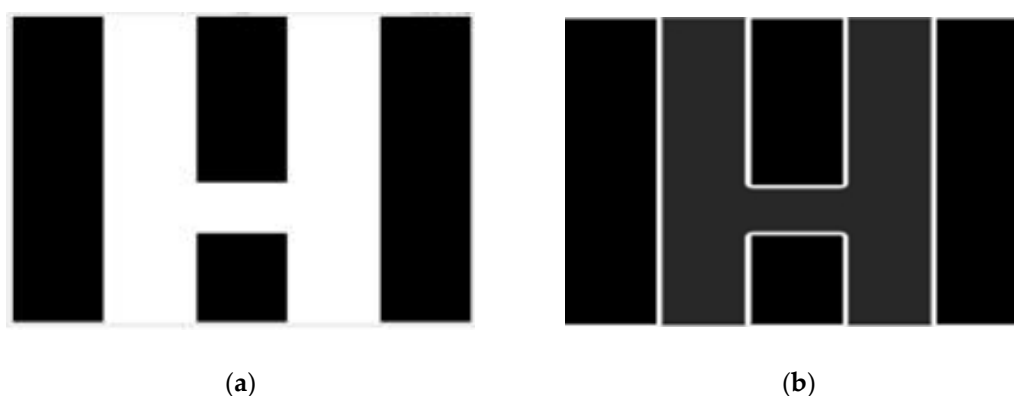
Figure 6. High-pass filtering of IDT local images with high-pass filtering: (a) partial diagram of IDT; (b) after filtering the graph by Gaussian high-pass filter.
