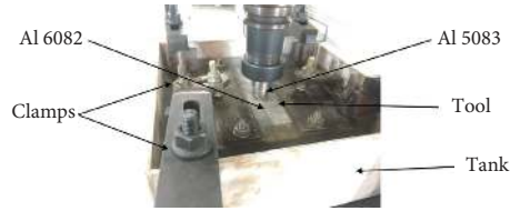
FIGURE 1: Submerged FSW set-up.
