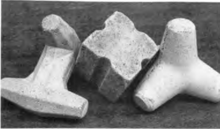
FIG.5 PHOTOGRAPH OF STRENGTH-SIMULATED MODEL DOLOS , CUBE D'ANTIFER AND TETRAPOD
