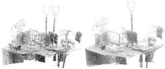
Figure 10: Illustration of the proposed ICP optimal variant for the TLS dataset, colored using ambient occlusion. Left: before registration. Right: after registration. No shift can be noticed.
