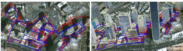
Figure 1: The Urban Canyon effect: In red, the GPS captured path. In blue, the actual path.
