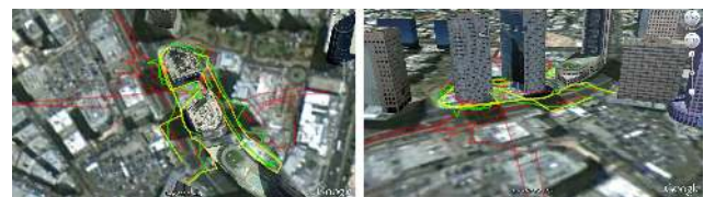
Figure 5: Improved Position: Left: above view. Right: 3D perspective view. In red, the path computed by a 1Hz fastrax GPS with an average error of 31 meters and max error of 180 meters; In green, the refined position with an average error of 4 meters and max error of 11 meters; In yellow, the actual path.
