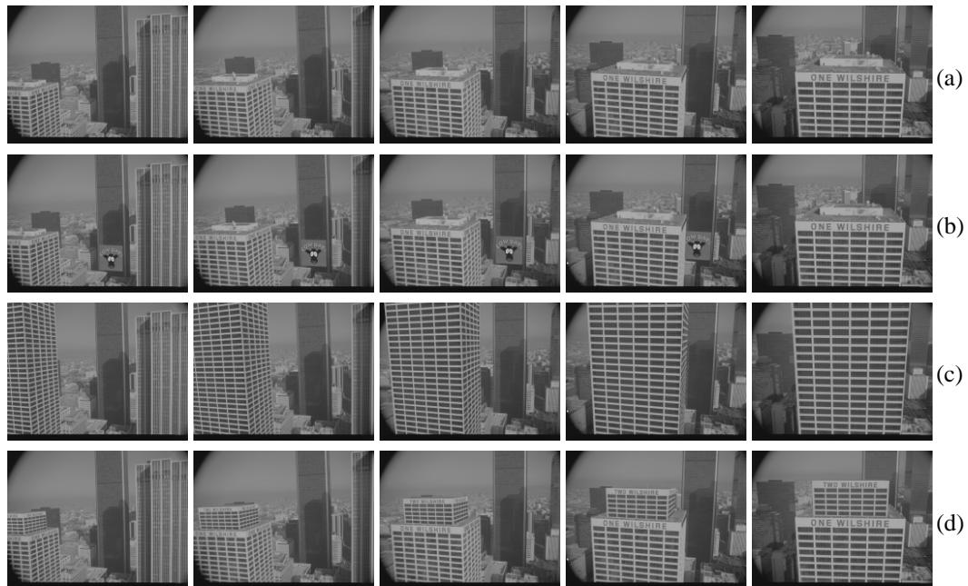
Figure 1: Typical AR tasks: (a) Five frames (between frames 70 and 220) from the Wilshire sequence. The images are 1024 \times 768 pixels. (b) Plane augmentation with occlusion —the ‘Cowdays’ logo is added to the far building and occluded by the sides of the foreground Wilshire building. (c) Plane extrapolation —the sides of the foreground “One Wilshire” building are extended. (d) 3D augmentation —an extra storey “Two Wilshire” is added to the top of the Wilshire building.
