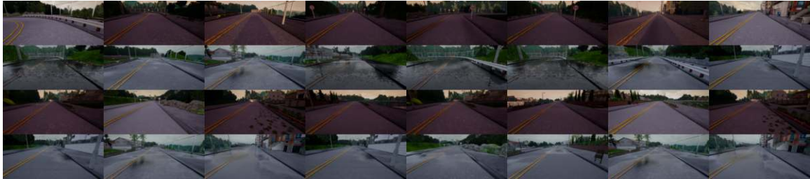
Figure 5.20: Source domain image samples and its corresponding aligned target domain images. The first and third rows are sunset environment images (source domain), the second and fourth rows are nearest neighbor images in the rainy environment (target domain).
