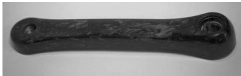
Figure 4. Natec pedal crank made with rCFRCs (desired characteristics: specific stiffness and equivalent mass to the classic one 185 g)
