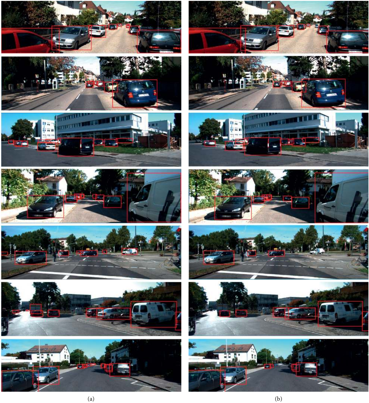
FIGURE 7: Detection results of the proposed method (a) and the original Faster R-CNN framework (b) on the KITTI validation set. As shown, the proposed approach can detect more small vehicles and avoid removing positive vehicle proposals unexpectedly (shown in the first row and the third row) compared to the original Faster R-CNN.
