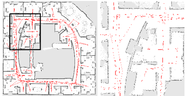
Fig. 3. Intel Lab , The robot starts in the upper part of the circular corridor, and runs several times around the loop, before entering the rooms. On the left, map generated with 15 particles. On the right a particular showing the accuracy of the map in the loop closure point, the resolution is 1 cm.
