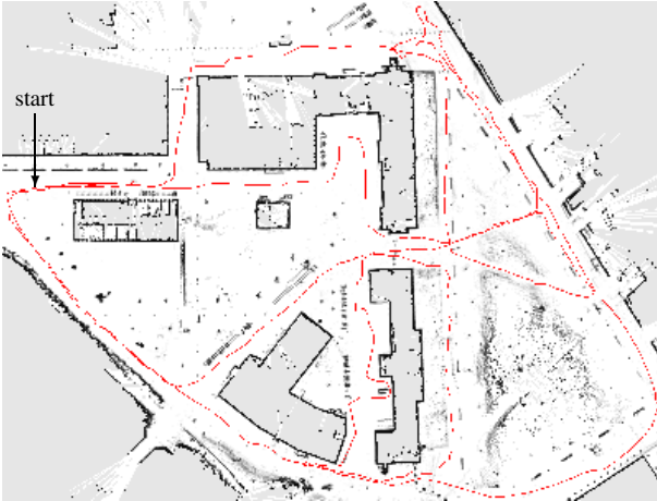
Fig. 4. Freiburg Campus The robot first runs on the external perimeter, for closing the outer loop. The internal parts of the campus are then visited. The area is 250 \times 250 m, and the overall trajectory is 1.7 km. Map generated with 30 particles.
