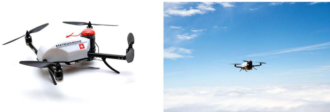
Fig. 4. Close-up of a Meteodrone. Equipped with an emergency rescue system it is allowed to fly under BVLOS (beyond visual line of sight) conditions up to 3 km AGL.
