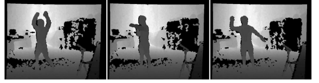
Fig. 1. Example of depth images of the actions (left to right) jumping jacks , punching , and throwing a ball .
