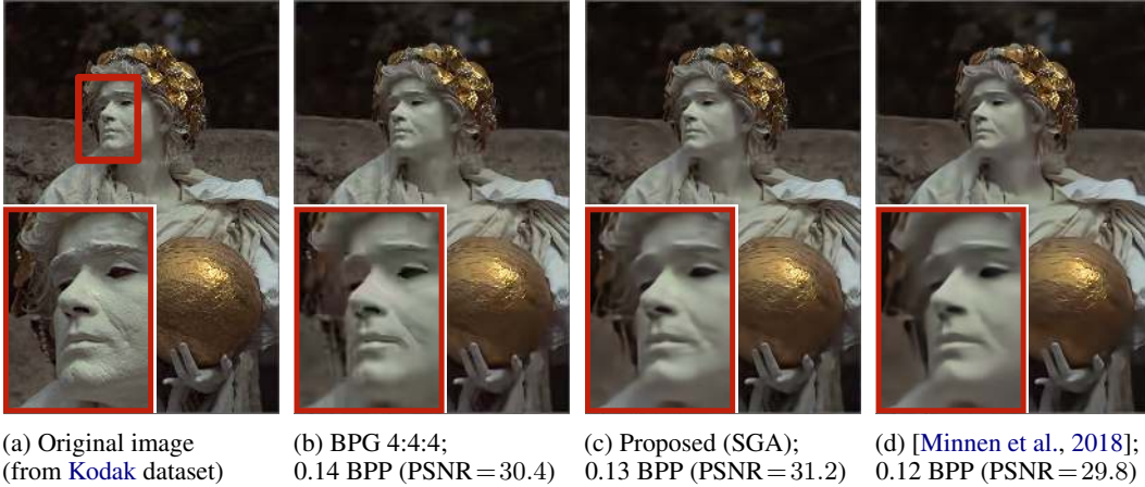
Figure 6: Qualitative comparison of lossy compression performance. Our method (c; [M1] in Table 1) significantly boosts the visual quality of the Base Hyperprior method (d; [M3] in Table 1) at similar bit rates. It sharpens details of the hair and face (see insets) obscured by the baseline method (d), while avoiding the ringing artifacts around the jaw and ear pendant produced by a classical codec (b).
