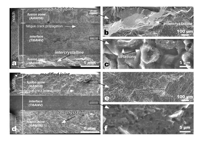
**Fig. 10** Fractographic differences after stabilization of fatigue crack propagation in the unmodified, a)-c), and the modified joint specimens, d)-f). The frames on the overall view mark approximately the respective area enlarged. Note the finer striations and the absence of intercrystalline fracture mode in the modified joint specimen.
