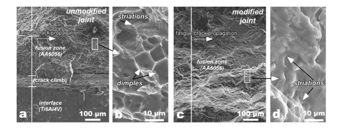
**Fig. 11** Fracture mode variation in very rapid fatigue crack propagation region at and after 25 mm in unmodified joint specimen, a)-b), and modified joint specimen, c)-d). The frames in a) and c) mark approximately the area enlarged in b) and d). Note the persistence of striations and the absence of dimples in the modified joint specimen.
