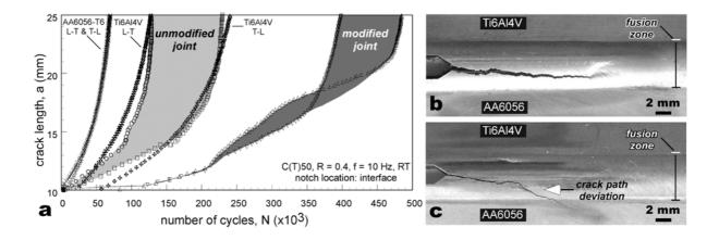
**Fig. 9** Improved resistance to fatigue crack propagation through the joint modification. The base material data in L-T and T-L orientations are shown for reference in a) and the crack path in the modified joint in b) and c). Note the crack path deviation *away* from the interface and into the Al-side in c).
