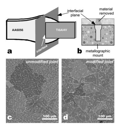
**Fig. 5** A schematic representation of the interfacial plane, a), and how it was reached for metallography, b). The microstructural differences in the interfacial plane, as imaged in the back scattered electron mode (material contrast) in SEM, are shown in c) and d) for the unmodified and the modified joint specimens. Variations in grain orientation are visible as the difference in gray colour, (specimens unetched).
