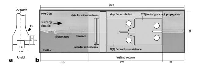
**Fig. 3** Dimensions of the machined U-slot used for the intake of Ti6Al4V sheet, a), and a typical laser beam welded coupon along with different specimens extracted, b). Locations of the fusion zone and the weld interface are also marked, (dimensions in mm).
