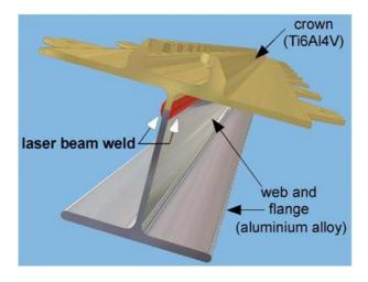
**Fig. 1** The passenger seat track as a laser beam welded dissimilar joint, (conceptual design after AIRBUS. The total height of the assembly is about 61 mm, the web height about 45 mm and the aluminium alloy flange width about 50 mm; drawing not to scale).
