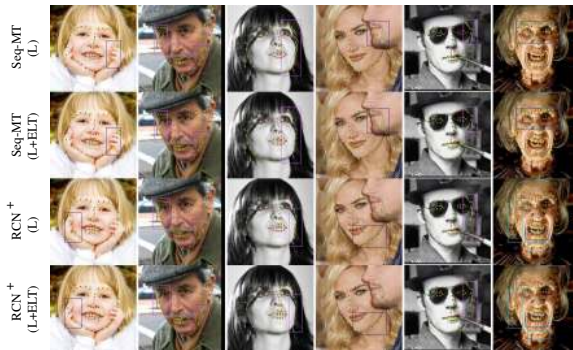
Figure 9: Landmark localization samples on 300W [27] test-set. The green and red dots show GT and model predictions, respectively. The yellow lines show the error. These examples illustrate the improved accuracy obtained by using the ELT cost. The rectangles show the regions that landmarks are mostly improved.
