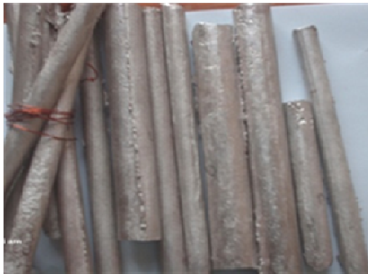
Fig. 4: Photograph of samples of the Al-Si-Fe/CSAp composite produced
