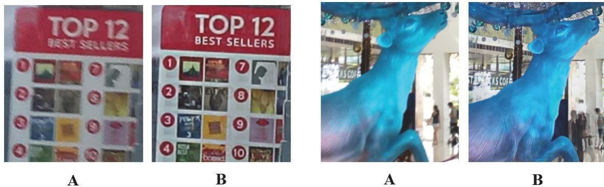
Figure 1: Sample HR images produced by the SR system with noticeable improvement. A: Bicubic interpolation. B: Proposed SR method.
