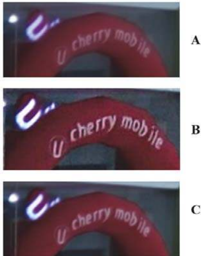
Figure 9: Unsharp masking illustration. A: LR image. B: LR image with unsharp masking applied. C: Resulting image after performing mean fusion. Observe that noise and other artifacts seen in B was suppressed, while having the edges preserved in C.
