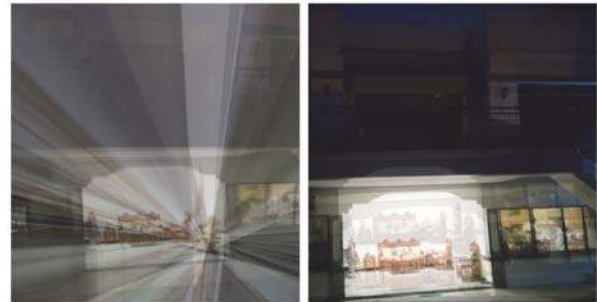
Figure 8: A: alignment using Perspective Transform Estimation. B: Best Alignment Technique. Aligning images with varying exposure values is a clear limitation of the MMISR system. This results in severe warping distortion only if (A) was applied. Misalignment and warping distortion is reduced if (B) was applied.
