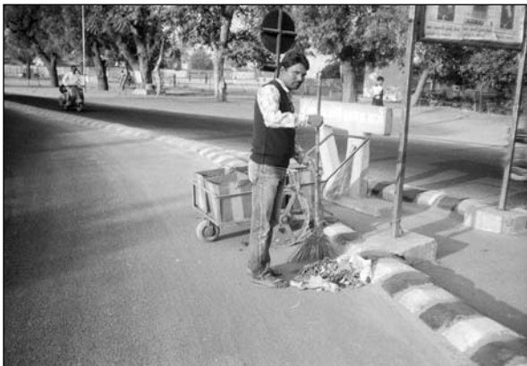
This street sweeper's containerized handcart is equipped with a handle at navel height plus a long-handled broom.
